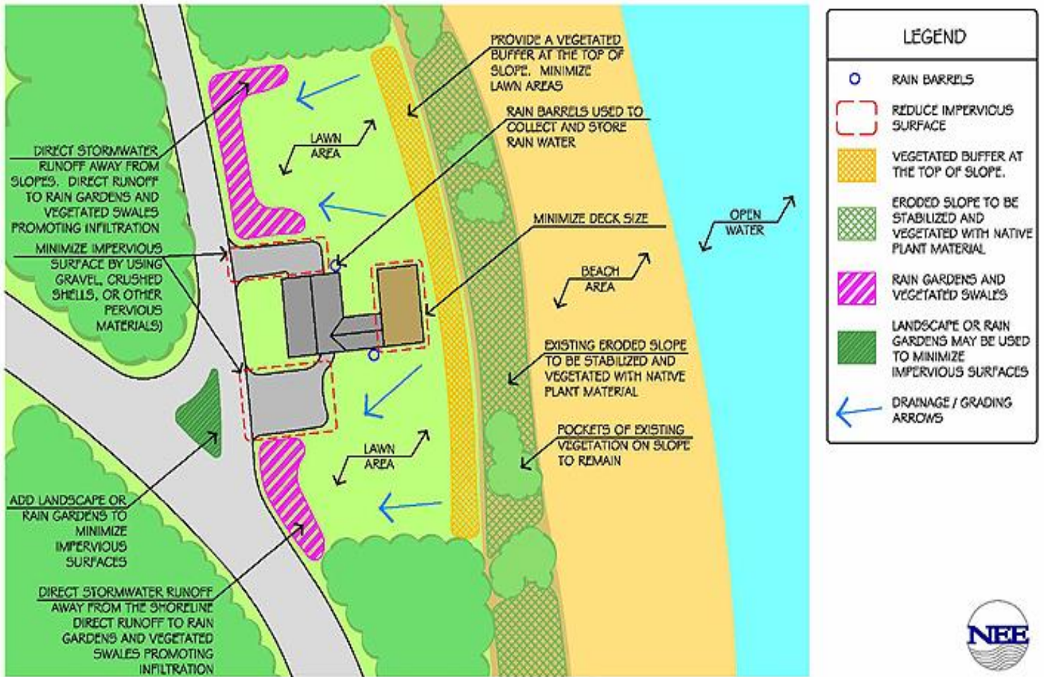
This figure demonstrates how a typical coastal property could be modified to reduce runoff and where appropriate runoff control techniques could be sited. (Graphic: New England Environmental, Inc.)
