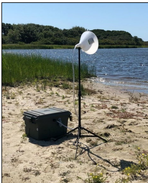
Figure 2-1. Glass fiber filter ASD showing filter cassette installed in the intake funnel.
