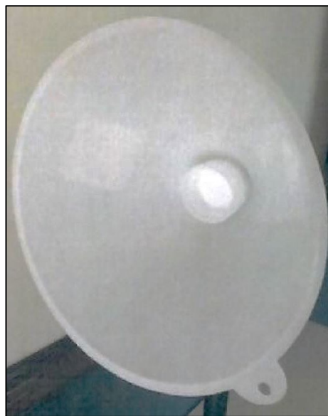
Figure 2-1. Glass fiber filter ASD showing filter cassette installed in the intake funnel.
